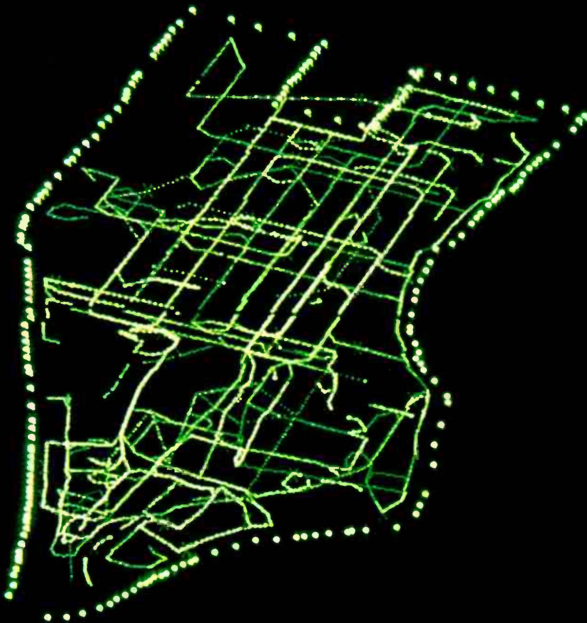
Simulated routes of several hundred vehicles of a personal rapid transit (PRT) system for mid- and lower Manhattan (from Central Park down). The computer simulation was carried out at the IBM Laboratories at Poughkeepsie, N.Y., and this picture was obtained through time exposure of the output cathode-ray tube display during the entire simulation. Requests for transportation from several hundred passengers' origins to their destinations were simulated through use of a random number generator. Each dot in the picture represents one vehicle with one passenger aboard, and the pickup and dropoff points for passengers are marked by X signs.
