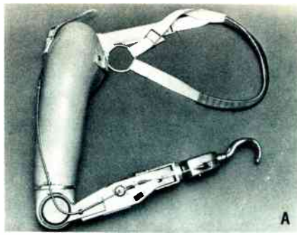
The "Boston Arm," an above-elbow prosthesis (A) uses the major electronic and mechanical components shown in (B). The electrodes are located in the upper arm socket and a nickel-cadmium battery pack is placed in the forearm of the prosthesis. Developed at Liberty Mutual Insurance Company's
