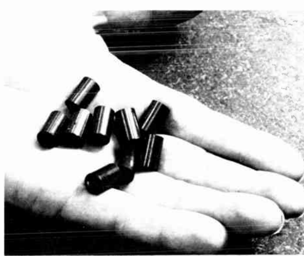
[1] Uranium oxide pellets like these, produced by Westinghouse, are used as fuel in pressurized water reactors (PWRs). When the fuel assemblies containing such pellets are placed in the reactor's core, each pellet can produce more energy than that produced by one tonne of coal.
