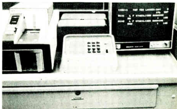
FIGURE 9 (below). Application of the Vicom system in an automotive plant. Display gives real-time data from product inspection.
