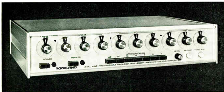
FIGURE 1. Front-panel controls permit the synthesizer to be set quickly.
