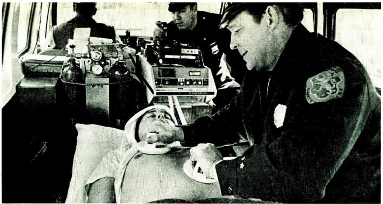
MOBILE TRANSMISSION OF ECG SIGNALS from emergency vehicle of the Nassau County Police Department is monitored by distant cardiologist who instructs police or other paramedics as to treatment and care of the patient. (Courtesy Pioneer Medical Systems)
