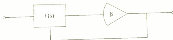
FIGURE 17. Basic single-loop feedback structure using one operational amplifier.
