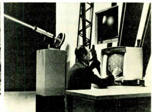
FIGURE 8. The IBM experimental optical transmission system at Expo '67. (Left) Aerial view of the communication path of the invisible infrared light beam (color overlay) used to transmit stock quotations from the Montreal Stock Exchange to the television display in the Canadian Pavilion almost 3 km away (link A) and two-way data/video (link B) from the IBM System/360 computer in the Canadian Pavilion to the IBM 2250 graphic display terminal at the Man-the-Producer Pavilion almost a kilometer away. (Below) Receiver unit reconverts light signals into electric impulses for display on the IBM 2250 terminal at the right.
