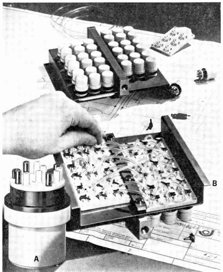
FIGURE 17. A plug-in fluidic NOR logic element based on the impact modulator principle (A) and an example of its assembly technique (B). (Courtesy of Johnson Service Company)
