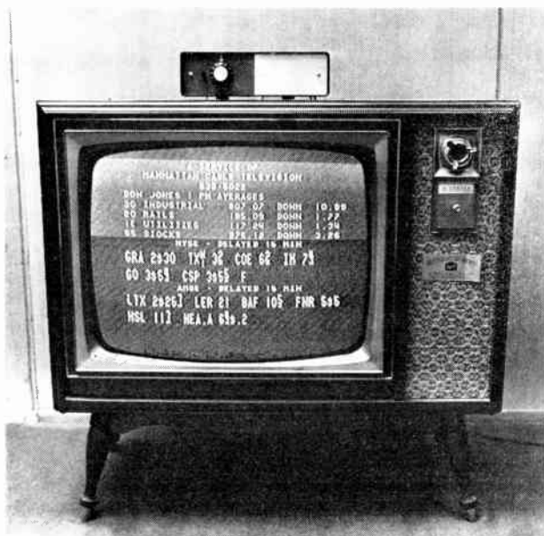
FIGURE 6. A typical service of cable TV picks up information directly from teletypewriter or stock market quotation service.
