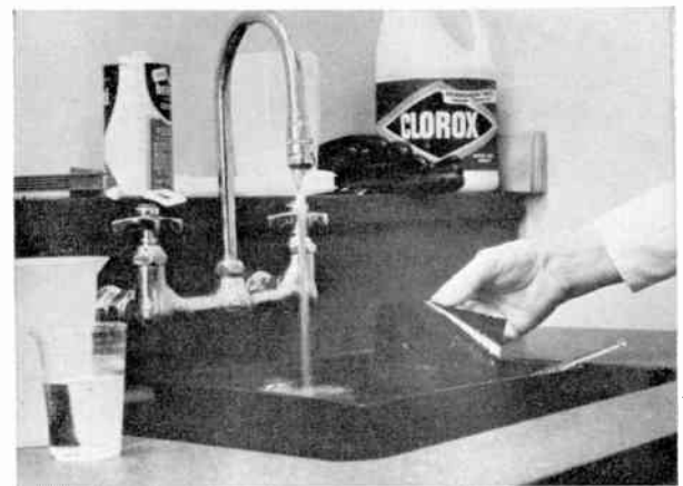
FIGURE 8. After being developed, material is washed in flowing warm water to clear printing areas of emulsion.
