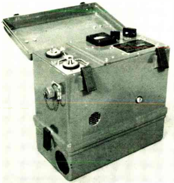
FIGURE 10. Exploratory development model of 60-watt hydrazine-air fuel cell.
