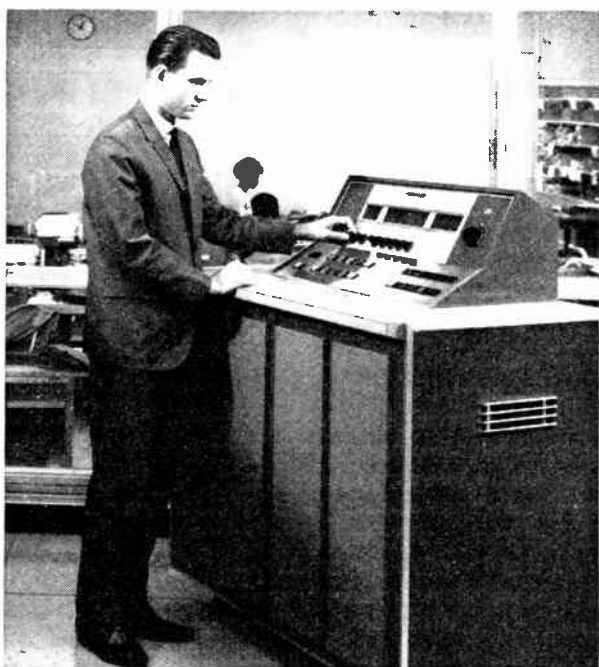
FIGURE 1. Control console of the Graphic Arts Composing Equipment (GRACE) system, installed by the National Library of Medicine in 1964 to serve as part of its publications subsystem. This photocompositor operates at a speed of 3600 words per minute.
