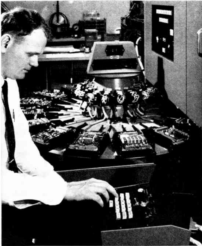
COMPARE system (see Session 4B) achieves automated troubleshooting analysis of the infrared signatures of electronic assemblies.
