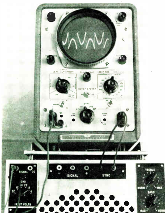
FIGURE 1. Aural and visual indication of the residue of a square wave after aural indication that the fundamental has been subtracted out.
