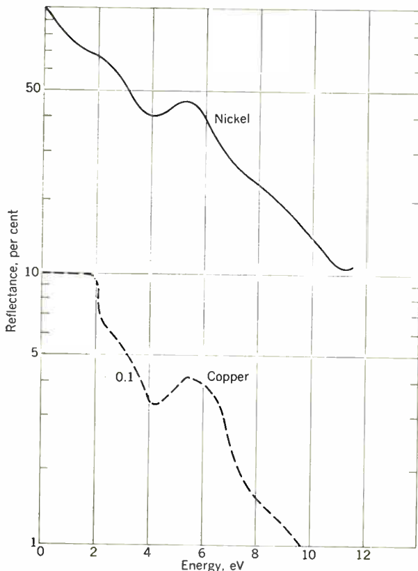
Fig. 16. Spectral dependence of the reflectance of copper 6 and nickel. (From Ehrenreich, Philipp, and Olechna 8 )
