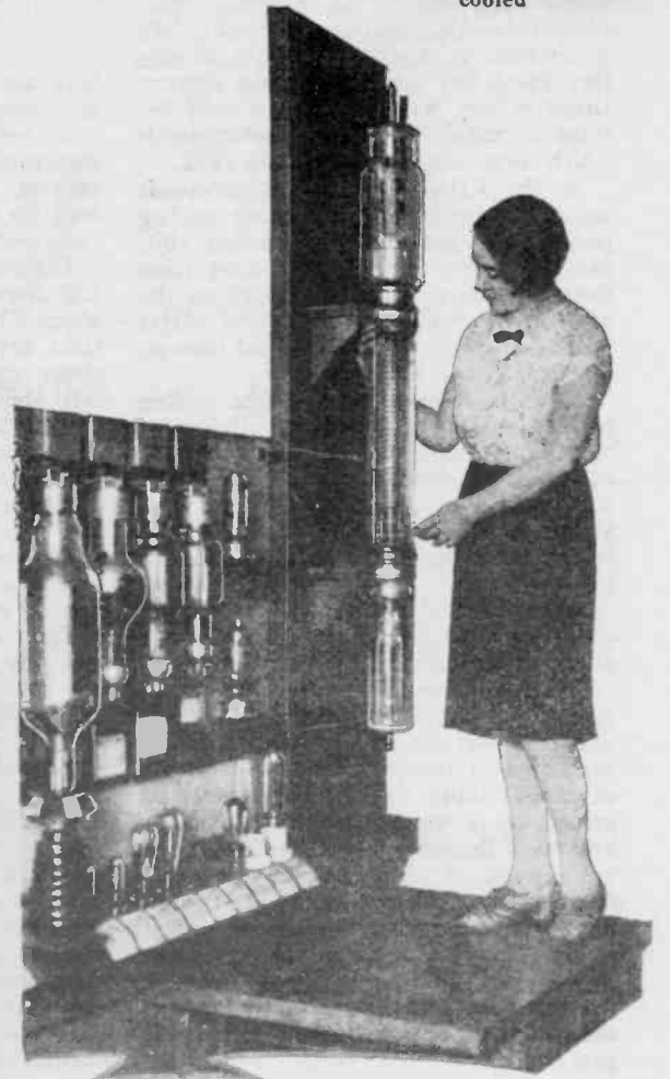
A W-220 tube is 72 inches in height, has a diameter of 8 inches and weighs 60 pounds. It has a capacity of 200 kilowatts and is water-cooled
