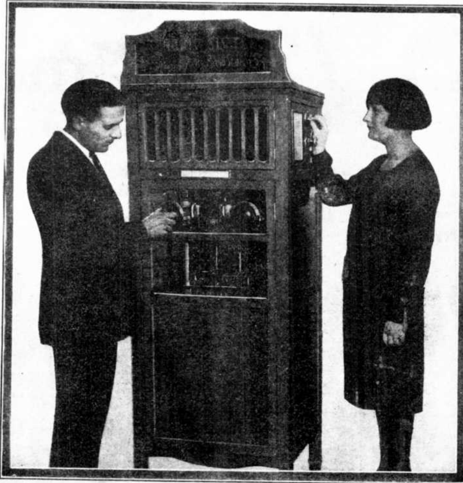
When a nickel is dropped in the slot, your favorite radio station can be tuned-in by the two dials on the front of the cabinet.
