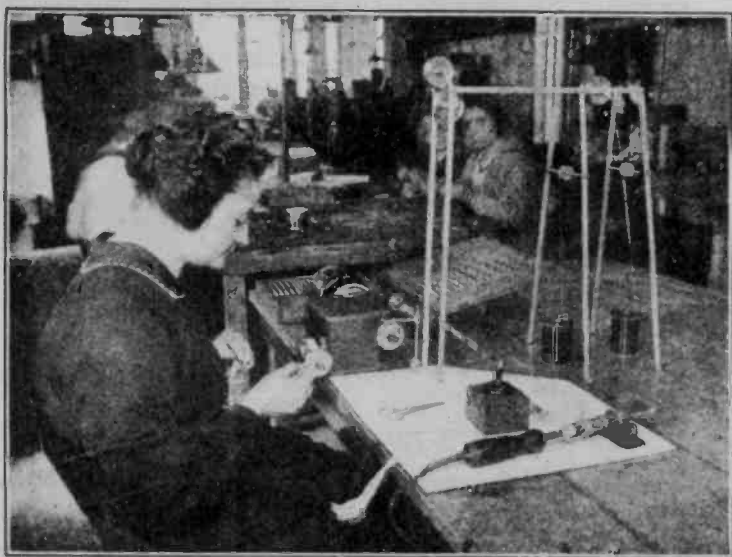
Left: These Machines Wind a Complete Bobbin in Less Time Than It Takes to Tell It; 3,500 Turns of Wire Per Minute Are Put in Place. A Special Counting Device Tells the Operator When the Proper Number of Turns Are Placed. Right: This Expert Mechanic Is Grinding the Pole Faces of the Magnets. Great Care Must Be Taken as the Removal of a Hairs-Breadth of Metal Too Much, Seriously Affects the Receiver's Operation.
