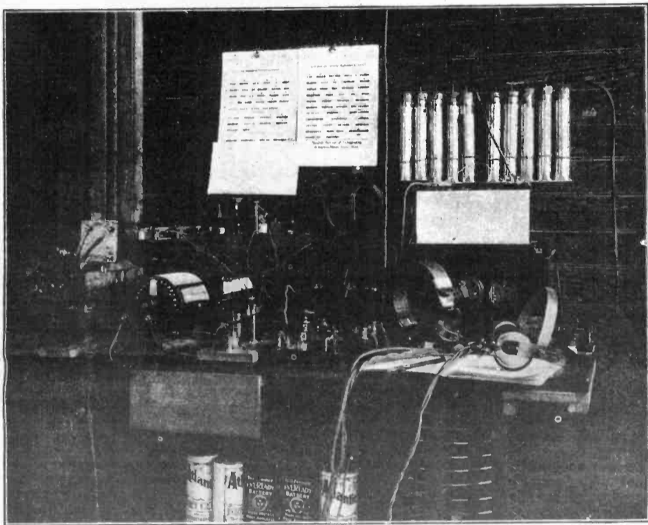
A typical amateur station of the 1912 type. Note the numerous detectors and the variable condenser on the extreme left. The glass tubes on the wall constituted the high tension sending condenser.
