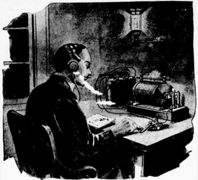
DeForest noted the change in brilliancy in a Welsback gas burner when his spark coil was in operation giving him the idea for the Audion.
