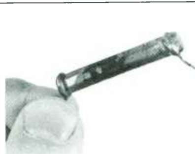
The overheated burned resistor was replaced with a new one of the proper value. Finding problems like that up front eases troubleshooting later.
