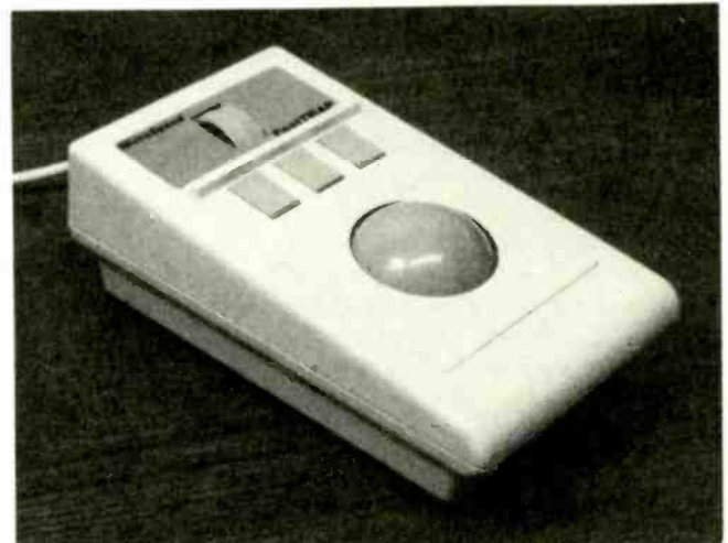
The FastTRAP is nearly identical to the PC-Trac, but adds a vertically oriented trackwheel. The trackwheel may be used for 3-D CAD work or for emulating various keystrokes in other programs—simulating PAGEUP and PGDN, for example.
