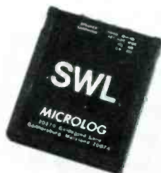
An SWL -equipped Commodore 64 or 128, when tied to a ham station can receive, decode, and display both Morse Code and radioteletype (RTTY) signals.
