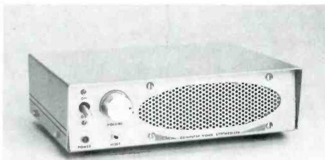
The prototype was housed in a home-made cabinet made from aluminum sheet metal. If you choose not to go to so much trouble, there are many ready-made cabinets on the market.
