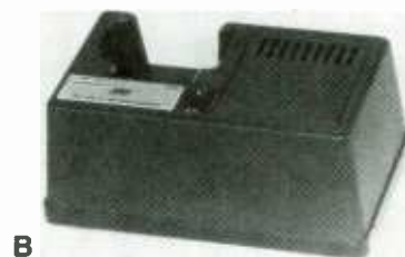
Fig. 5—Shown here are two popular accessories for the 2-meter handheld transceiver. The accessory shown in "A" is an MFJ speaker microphone, which incorporates both microphone and loudspeaker functions in the same case. The accessory shown in "B" is the MFJ charger stand.
