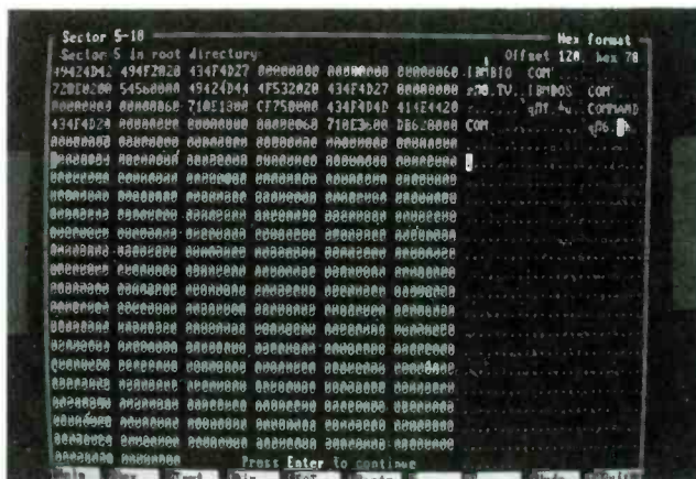
The Norton Utilities chief claim to fame is the ability to “unerase” (or recover) files, but they are also useful for byte-level disk editing, and many other things as well.
