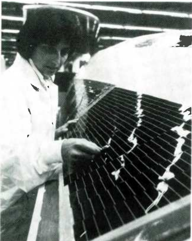
A critical construction step was to bond the solar cells to the Sunraycer's body. 7,200 solar cells are mounted on 90 square feet of the aerodynamic, domed surface. The work was performed at Hughes Aircraft Co. facilities in California.
