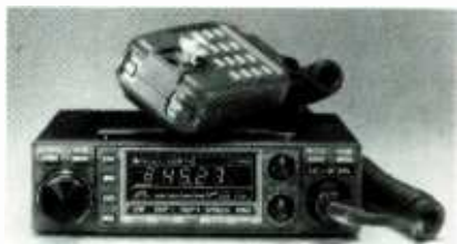
Fig. 3—Shown here is a typical mobile rig—the Icom IC-27A. Note the size relative to the hand-held microphone. The microphone not only serves the microphone function, but also contains the Touchtone pad needed to use the autopatch, and up/down switches to change the set's operating frequency.
