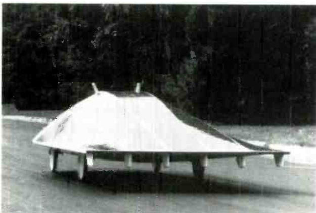
A loser's view of the Sunraycer "easing on down the road." Two protuberances on top give it an "out-of-space" appearance, but they serve to stabilize the racer in strong cross winds.
