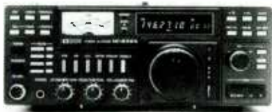
Fig. 2—The rig shown here is an Icom Model IC-727A base station intended for home use, and is typical of all-mode rigs, which allow the user to select either CW, AM, SSB or FM modes. Like most modern ham rigs, it offers memory as well as VFO tuning.
