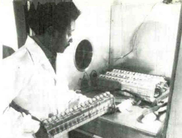
The Sunraycer's silver-zinc battery cells are put to the test in an environmental chamber that produces the worst-possible conditions a vehicle could possibly experience in Australia.
