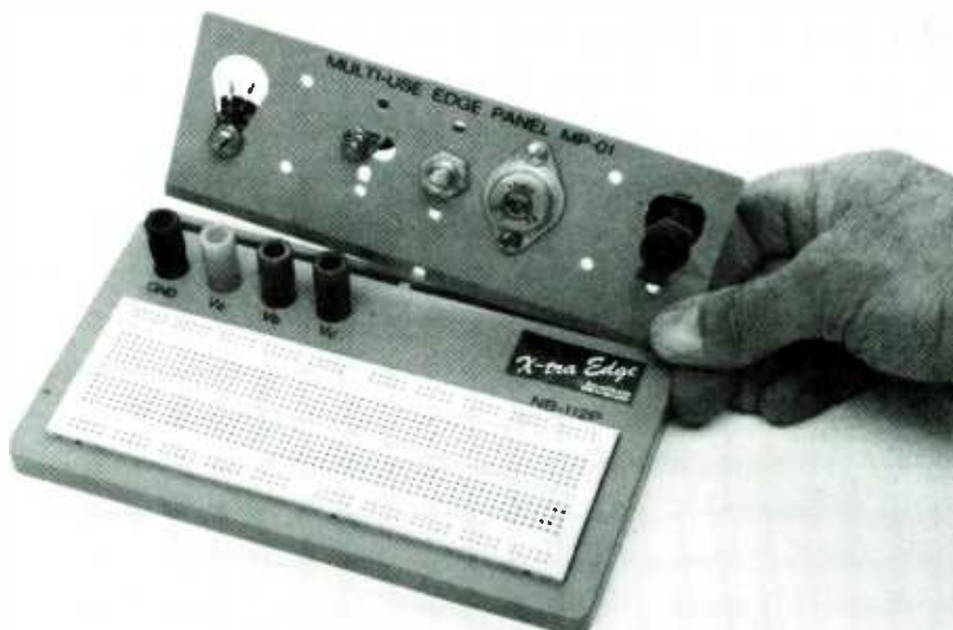
The edge panel simply slips into a slot on the rear of the breadboard's base. No hardware of any kind is needed to keep it in position. Notice the small keyway (center of the bottom edge) that keeps the panel from sliding to the side.
