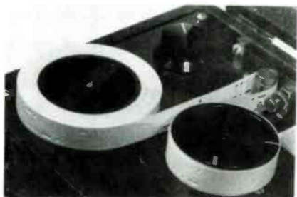
This close-up of the top panel shows the transport system for perforated tape.
