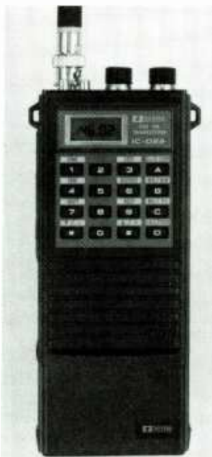
Fig. 4—Typical of handheld rigs, the Icom Model IC-02A is self-contained with receiver, transmitter, and autopatch Touchtone pad; and offers several watts of RF output power.
