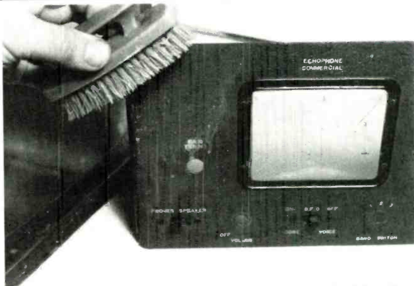
The paint on the front panel/cabinet assembly became several shades lighter after removal of grime with ordinary hand soap and a soft scrub brush.
