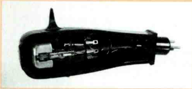
Later model G.E. cartridge as found mounted in Garrard RC-88, bearing the designation VRII , takes the same replacement armature as original cartridge.
