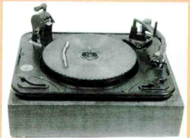
The Garrard RC-88 changer, with a short spindle accessory for automatic turntable mode is installed. Longer spindle for record changer mode is displayed on turntable mat.
