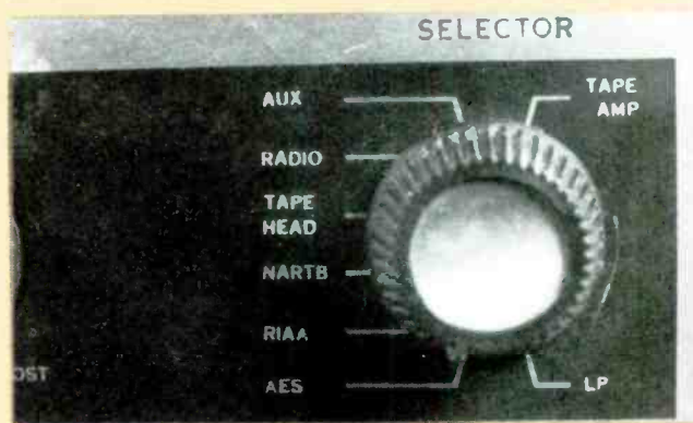
The input selector on this mid-1950's hi-fi amplifier includes four magnetic cartridge equalization positions.
