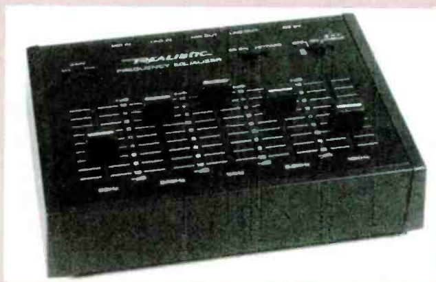
Radio Shack #32-1115 5-band mono equalizer. Even a simple unit such as this unit will be amazingly effective in adding richness and depth to your old audio tracks.
