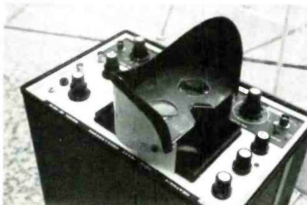
The center of each lens should be directly over its corresponding flat trace at zero volts. The viewer can be moved over any portion of the wave forms in the X direction.
