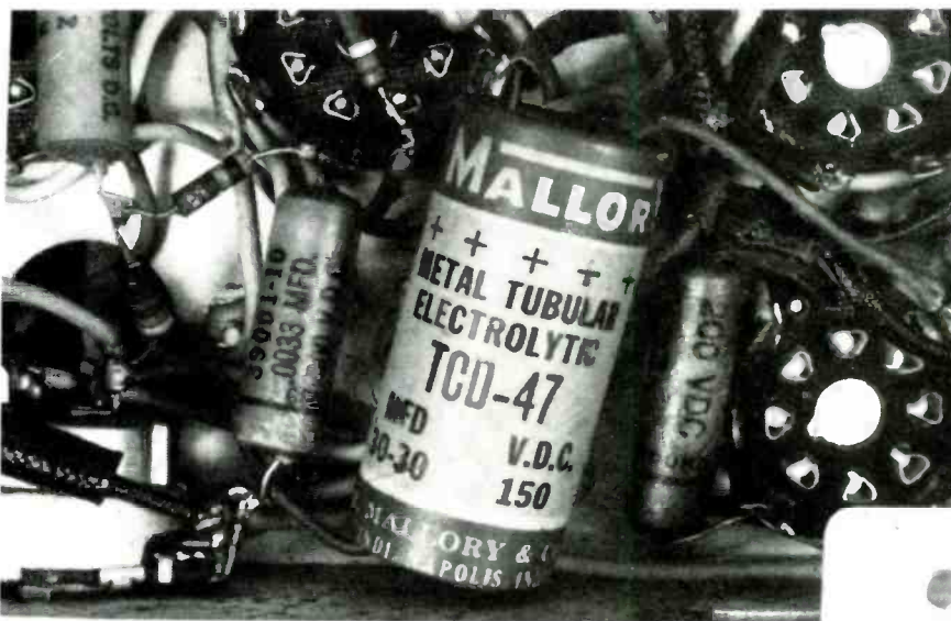
This small 1940's AC/DC table model has a cardboard-covered 2-section electrolytic capacitor mounted under the chassis.
