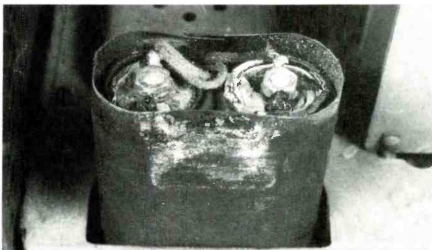
Check out this capacitor can from a 1920's era radio with cover removed. Inside are two wet electrolytics. If you look very closely, you'll notice corrosion on the cans, which was caused by electrolyte leakage.
