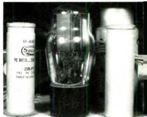
The rectifier tube in this 1930's radio is flanked by two individual electrolytic units in aluminum cans.
