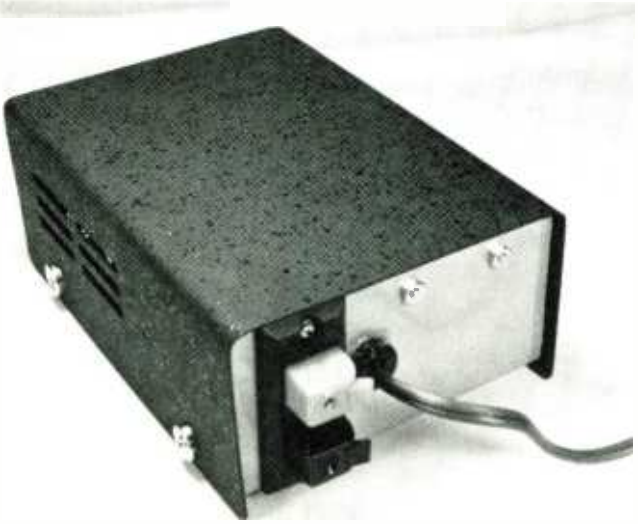
The two screws in the upper right are used to hold the buzzer in place. The strip on the left is used to connect the long zip-cord from the remote sensor to the remote power-supply box. Note that the AC line cord is fastened.
