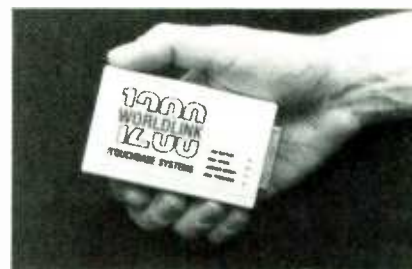
This tiny battery-operated modem, which is intended for portable computers, isn't much larger than a few fingers, yet it packs the full complement of Hayes commands. It ran from every standard and conventional software package we tried.
