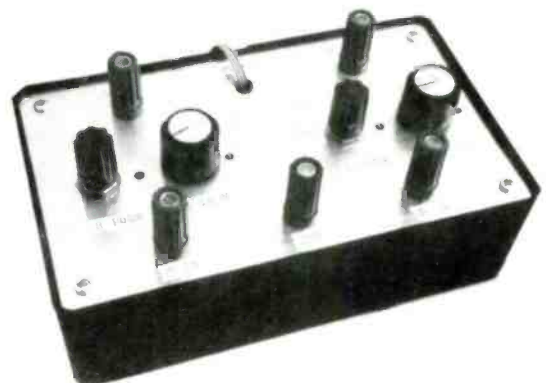
Typing labels on sticky-backed paper gives the project a neat, finished look. If you use that method of labeling be sure to place clear tape over each label. That is to keep the ink from smearing on the paper's smooth finish.
