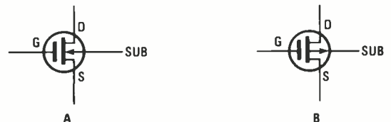
Fig. 31—The generally-used schematic symbols that are used for depletion mode MOSFET's: A) N-channel; B) P-channel.
