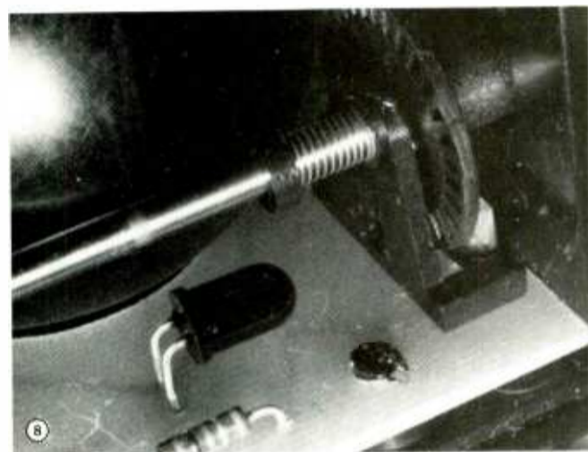
Take the cover off a trackball and it really looks different (top). The ball actually rotates two shutter mechanisms. A close look at a shutter (bottom) shows that it provides an on-off switching action by interrupting the light from an infrared LED that falls on a photodetector.
