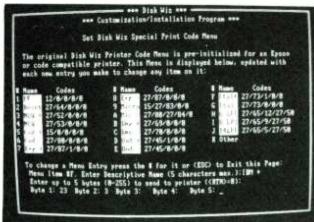
Fig. 1—The Disk Wiz customizing program allows you to pre-program up to 20 printer control codes that are sent to the printer at the touch of a single key. At the bottom, the screen shows we want to change The "Ital +" to read "IBM +," and we will program a new printer code for IBM of 23/3/0/0/0.
