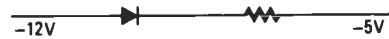
Fig. 7—Bias with only negative voltages applied. No current flows because the cathode is positive to the anode.
