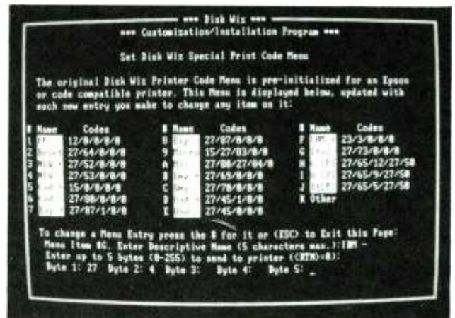
Fig. 2—The first change is made! Note that item F now reads "IBM +," and that the printer code is changed. The bottom of the screen shows the programming for "IBM -" is ready for entry.
