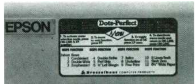
The final step in the retrofit is to apply the decal (label) that shows the programming provided by the printer's on-line, LF and FF panel controls.
