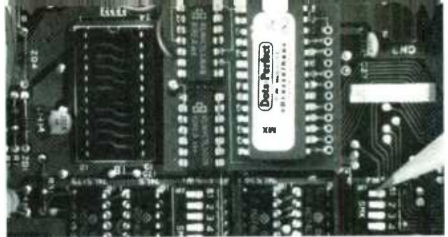
The pencil indicates the location of the 8-position DIP switch, which must be set for the normal power-up defaults.
