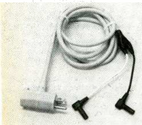
The adapter is simply a 5-ft. harness having a plug and receptacle on one end and hooded banana jacks on the other.
