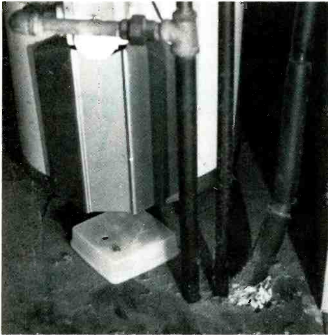
The Waterbug can be placed anywhere that flooding is likely to occur; under a water-heating unit or in the laundry room, etc.
