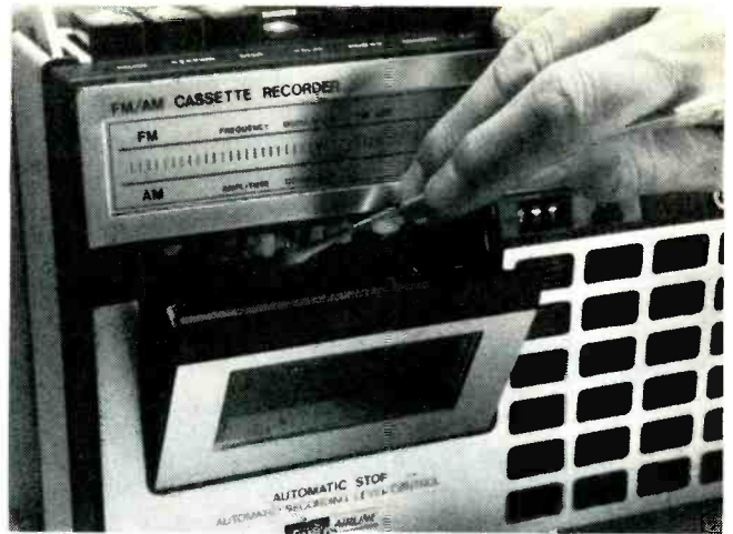
A dirty tape head can cause weak sound, distortion, or a noisy stereo channel. Check the erase head for excess oxide that may prevent full erasure of a previous recording.
