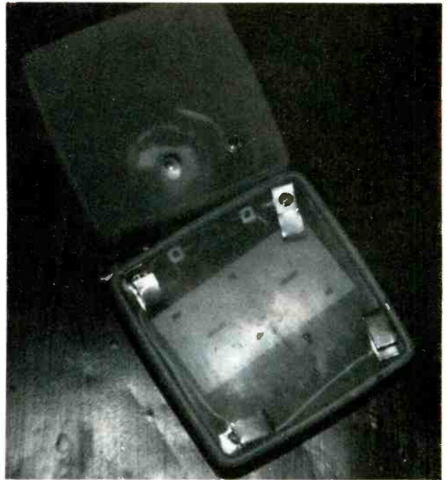
An ordinary plastic sandwich box—which can be found at drug and variety stores, or supermarkets—is used to house the series-connected batteries and components that make up the circuit.
