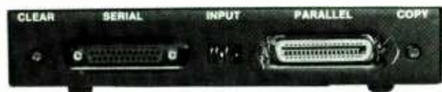
The input side of the Universal Printer Buffer has serial and parallel connectors, a DIP switch for setting serial communications parameters (baud rate, etc.), and Copy and Clear switches.
