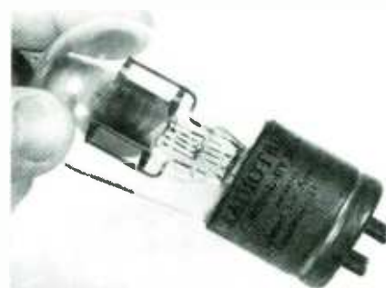
The UV-201 was one of the first two receiving tube types produced by RCA.
