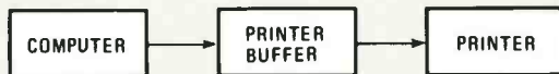
Fig. 1—A printer buffer is little more than a block of memory positioned between your computer and its printer. A commercial printer buffer may have as little as 8K or as much 1 megabyte (or possibly even more!) of memory.
