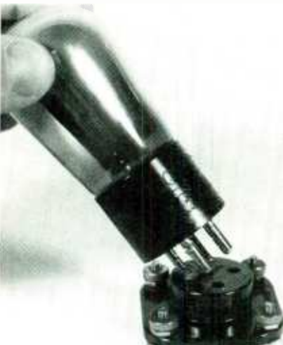
A '01-A-type tube with UX-style base. Elongated contact pins sit in matching socket holes.
