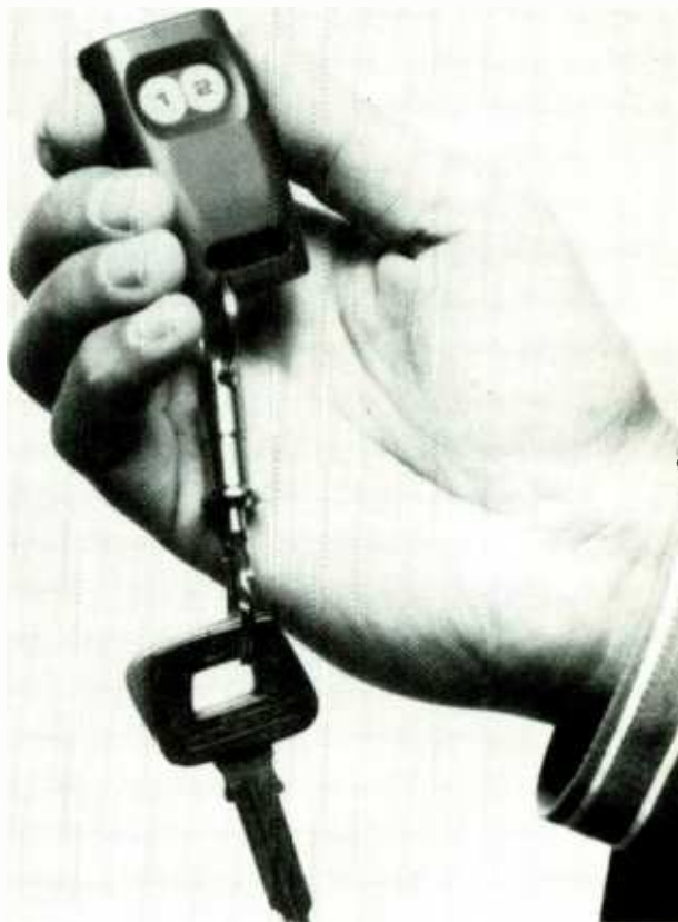
Remote control transmitters that will open car doors and the trunk from almost 50-feet away are small enough to mount on a key-fob. This one has two buttons for control of two vehicles.
