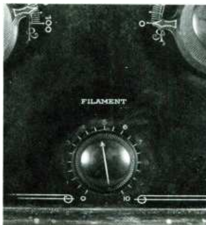
The filament-voltage rheostat (center knob) was standard equipment on early battery-powered sets.
