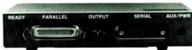
The output side of the Universal Printer Buffer has serial and parallel connectors, a DIP switch for setting serial communications parameters (baud rate, etc.), a power jack, and an LED that indicates status (ready and number of copies).
