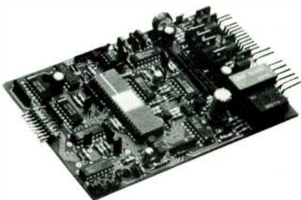
Although the the most basic auto-alarms need only a noisemaker, a latching relay, and a few switches, the control box of a computerized alarm system usually has a printed-circuit board jam-packed with transistors, integrated circuits, and a microprocessor.
