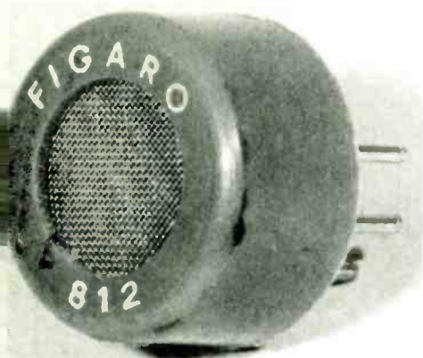
The gas sensor used as the basis of the Toxic-Gas Alarm fits neatly into any standard 7-pin vacuum tube socket.
