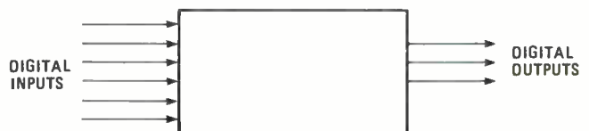
Fig.1—When we are interested primarily in input and output signals, we can use a "black box" to represent some kind of digital circuit, combinational or sequential, that processes the inputs to generate new outputs.
