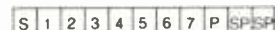
Fig. 1—The conventional ASCII terminal uses 11-bits per character at 110 baud; 10 bits at 300 baud and higher transmission rates. At a 300 baud rate (or more) the second stop bit is eliminated.
