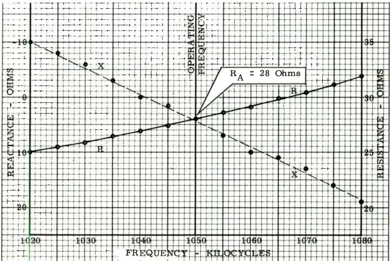
DIRECTIONAL COMMON POINT IMPEDANCE MEASUREMENTS
