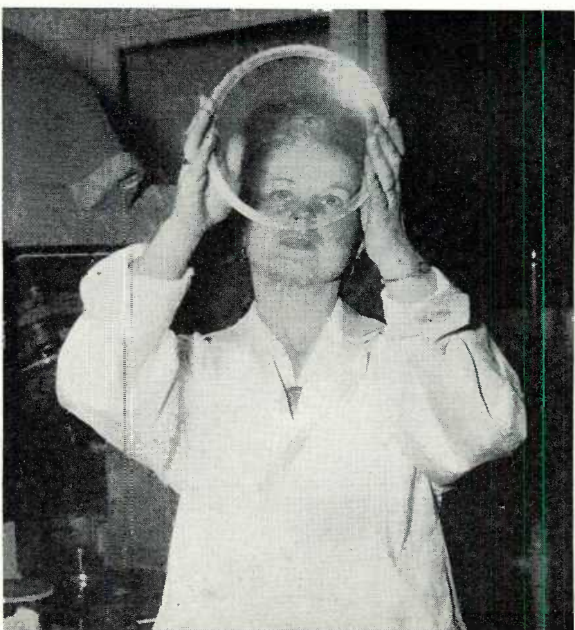
FIG. 5, LEFT. SINCE THIS IS THERMOPLASTIC MATERIAL, THE MOLDS MUST BE COOLED BY WATER CIRCULATION BEFORE THE LENS CAN BE REMOVED. FIG. 6, RIGHT. NO FINISHING PROCESS IS REQUIRED ON THE LENS SURFACE. THIS LENS WILL BE READY FOR OPTICAL CHECKING AS SOON AS A HOLE HAS BEEN CUT OUT AT THE CENTER
