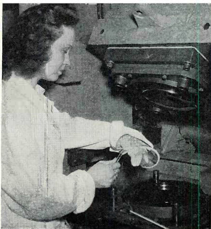
FIG. 3, LEFT. IN THIS OVEN THE PREFORM IS PLACED BETWEEN DISC ELECTRODES CONNECTED TO THE RF GENERATOR. THIS HEATS THE PREFORM EVENLY THROUGH. FIG. 4, RIGHT. THE HEATED PREFORM, NOW SOFT ENOUGH TO BE FLEXIBLE, IS INSERTED IN THE MOLDING PRESS, WHERE IT WILL BE FORMED, AS IN FIG. 1, INTO A PERFECT LENS
