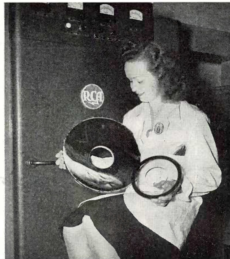
FIG. 9, LEFT. HERE IS THE BLANK SHOWN IN FIG. 7 AFTER THE ALUMINIZING PROCESS HAS BEEN COMPLETED. THE REFLECTIVE POWER IS MUCH HIGHER THAN THE RELATIVELY INEFFICIENT SILVERING OF ORDINARY MIRRORS. FIG. 10, RIGHT. A FINISHED REFLECTOR AND CORRECTING LENS, READY TO BE CHECKED BEFORE MOUNTING IN A RECEIVER
