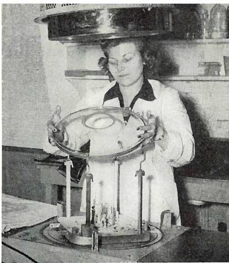
FIG. 7, LEFT. THE GLASS BLANK FOR THE MIRROR IS GROUND AND POLISHED ON STANDARD OPTICAL MACHINES, SINCE ITS SHAPE INVOLVES NO SPECIAL PROBLEMS. FIG. 8, RIGHT. THE BELL JAR AND PROTECTIVE SCREEN ARE LOWERED OVER THE GLASS BLANK, AND THE BELL JAR IS EVACUATED WHILE ALUMINUM IS DEPOSITED INSIDE THE BOWL
