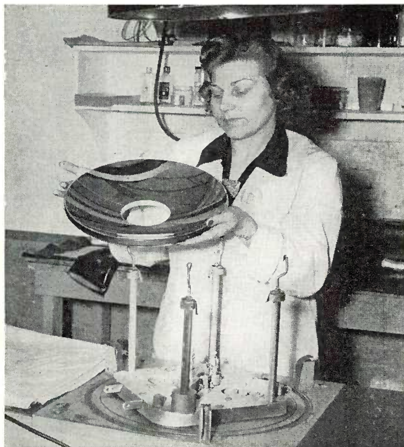
FIG. 9, LEFT. HERE IS THE BLANK SHOWN IN FIG. 7 AFTER THE ALUMINIZING PROCESS HAS BEEN COMPLETED. THE REFLECTIVE POWER IS MUCH HIGHER THAN THE RELATIVELY INEFFICIENT SILVERING OF ORDINARY MIRRORS. FIG. 10, RIGHT. A FINISHED REFLECTOR AND CORRECTING LENS, READY TO BE CHECKED BEFORE MOUNTING IN A RECEIVER
