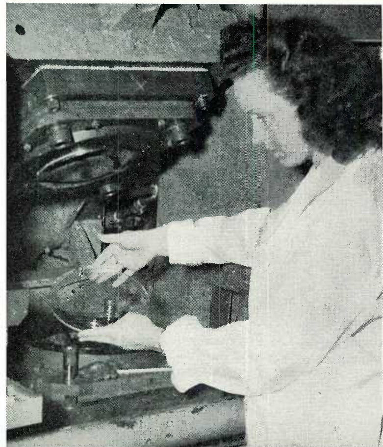
FIG. 5, LEFT. SINCE THIS IS THERMOPLASTIC MATERIAL, THE MOLDS MUST BE COOLED BY WATER CIRCULATION BEFORE THE LENS CAN BE REMOVED. FIG. 6, RIGHT. NO FINISHING PROCESS IS REQUIRED ON THE LENS SURFACE. THIS LENS WILL BE READY FOR OPTICAL CHECKING AS SOON AS A HOLE HAS BEEN CUT OUT AT THE CENTER
