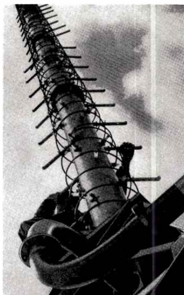
FIG. 13. ABOUT 3½ BAYS ARE VISIBLE OF A 5-BAY SIDE-FIRE HELICAL ANTENNA FOR UHF-TV
