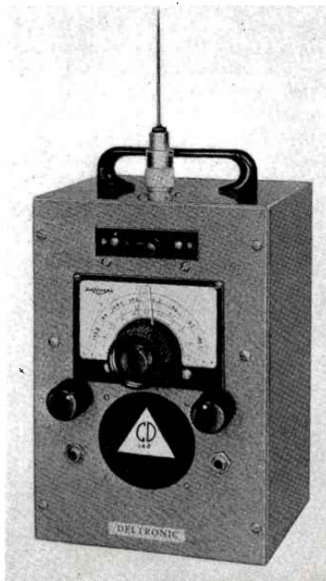
LEFT: PORTABLE AM UNIT HAS NARROW BAND TUNING. RIGHT: BUDELMAN RADIO IS BUILDING THIS VEST-POCKET AM RECEIVER FOR RADIO PAGING
