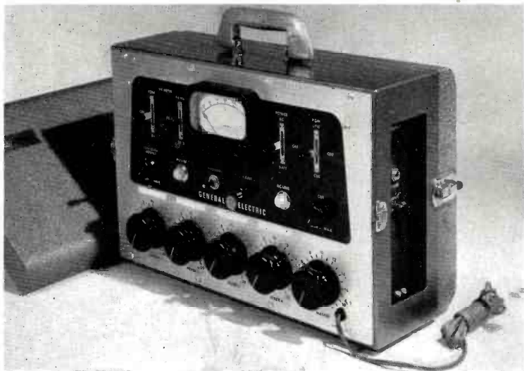
FIG. 3. THIS BROADCAST AMPLIFIER CAN BE EMPLOYED FOR REMOTE OR STUDIO APPLICATIONS
