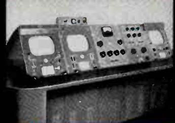
Similar setup with two camera control units (one live and one film, or two film), such as used in the RCA "Basic Buy" for TV.
