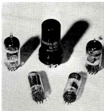
LEFT: ADDED HIGH-RELIABILITY GE TUBES ARE, LEFT TO RIGHT, 6L6072 (12AY7), 6L6136 (6AU6), 6L6137 (6SK7), 6L6135 (6C4W), AND 6L6201 (12AT7). CENTER: AVION INSTRUMENT COMPANY'S SUBMINIATURE TUBE AND CIRCUIT ASSEMBLY. RIGHT: BENDIX CONTROL UNIT FOR RADIO SYSTEM DISPATCHERS
