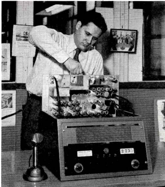
LEFT: NEW 60-WATT RCA DESK-MOUNTING EQUIPMENT FOR ADJACENT-CHANNEL OPERATION. RIGHT: JUNCTION BOX FOR SHIFTING TRANSMITTERS
