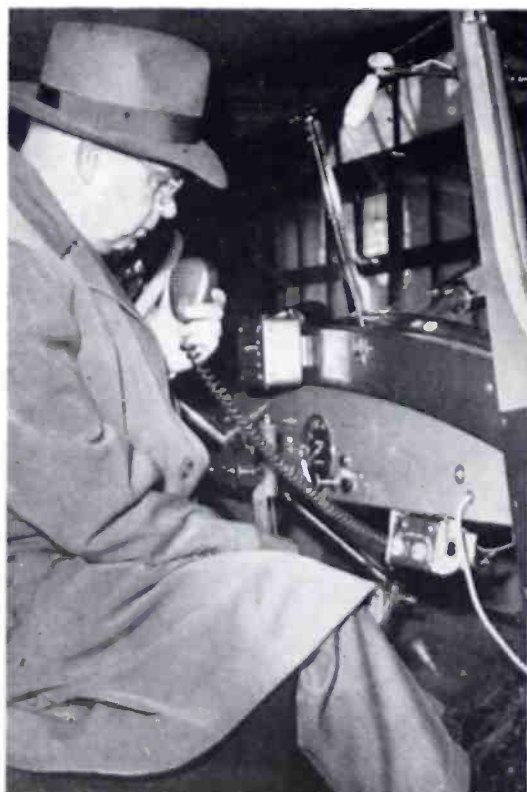
FIG. 8. FIRE CHIEF ANDREW JONES USING 2-WAY MOBILE RADIO EQUIPMENT WHICH IS MOUNTED ON RUNNING BOARD UNDER LADDER, FIG. 9
