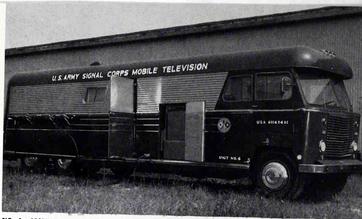
FIG. 8. RECEIVING POWER UNIT. THIS VEHICLE CONTAINS A 15-KVA. ENGINE-DRIVEN GENERATOR, TEST EQUIPMENT, SPARE PARTS, AND REELS FOR AUDIO, VIDEO, AND POWER CABLES
