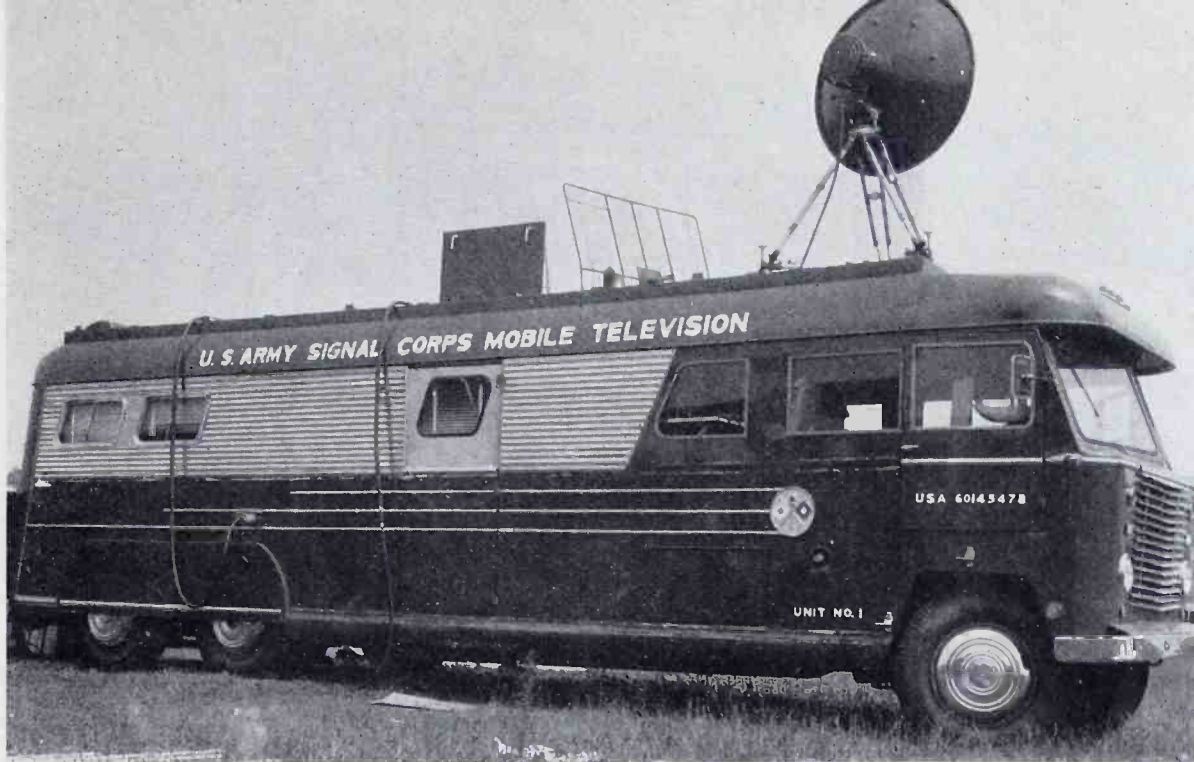
FIG. 1. TRANSMITTING UNIT OF THE CARAVAN. ROOF IS REINFORCED TO SUPPORT WEIGHT OF ANTENNAS, CAMERAS, AND OPERATORS, SO THAT IT CAN BE EMPLOYED AS A CAMERA PLATFORM
