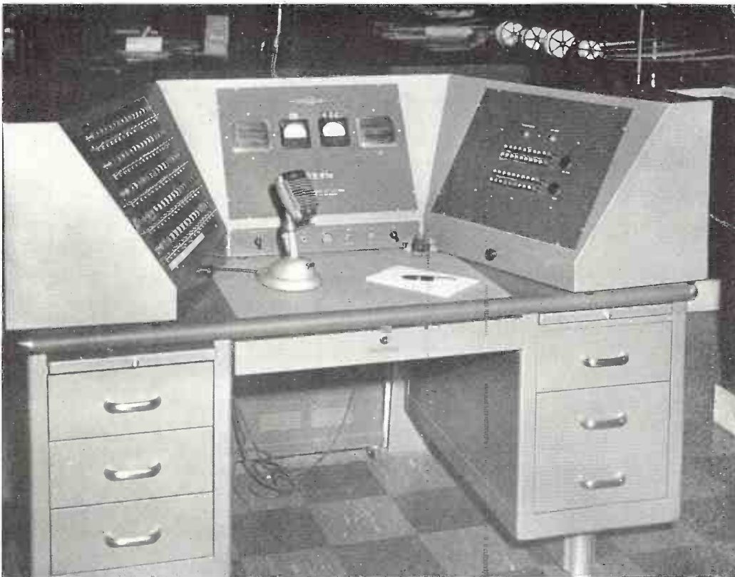
FIG. 4. LINK RADIO CONSOLE HAS CALLING BUTTONS AT RIGHT, IN-SERVICE LIGHTS AT LEFT
