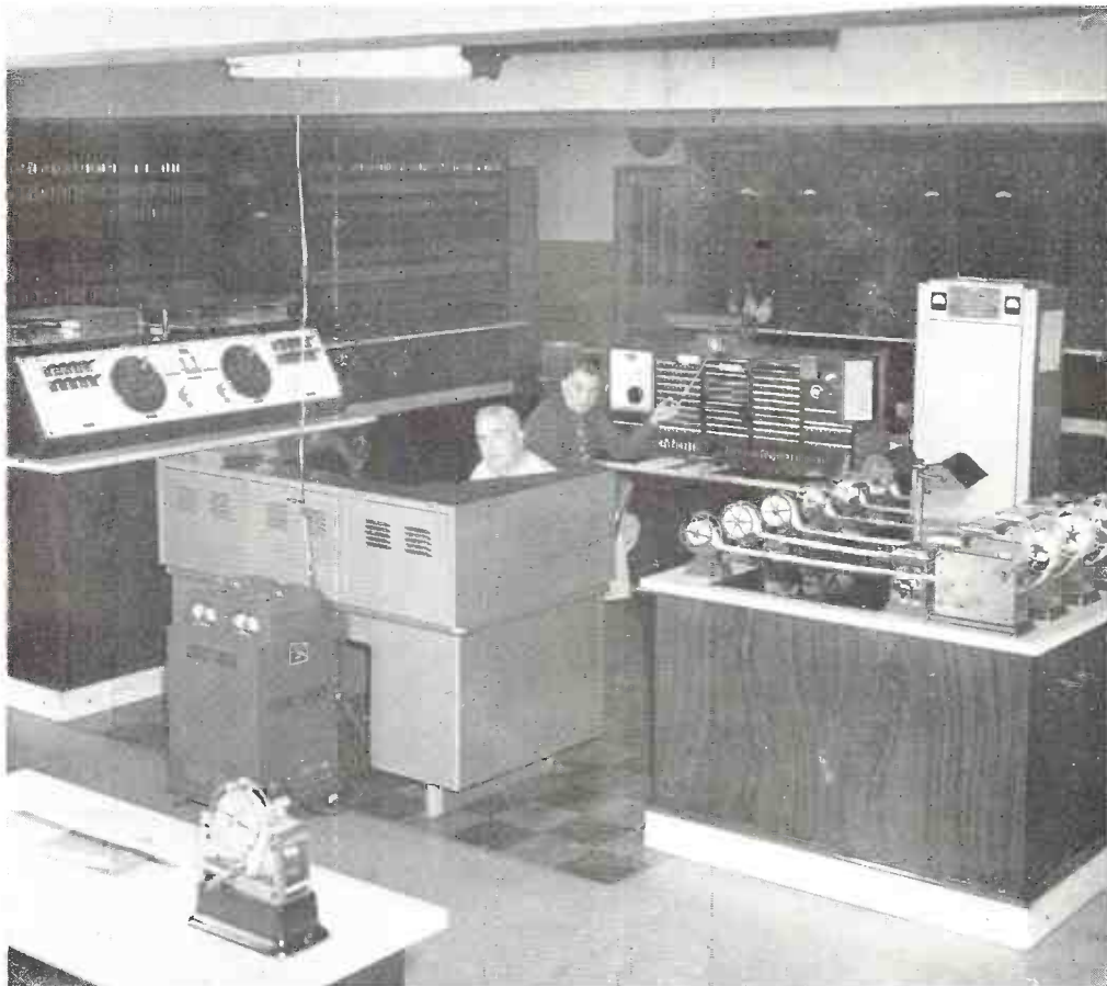
FIG. 2. THE RADIO CONTROL CONSOLE AT FIRE HEADQUARTERS TRANSMITS ALARMS OF FIRE TO THE STATIONS BY SELECTIVE RADIO CALLING
