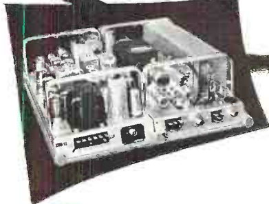
450-MC MOBILE RADIO EQUIPMENT (RADIO TRANSMITTER-RECEIVER TYPE 2210-ED.2 WITH CONVERTER TYPE 2581)
