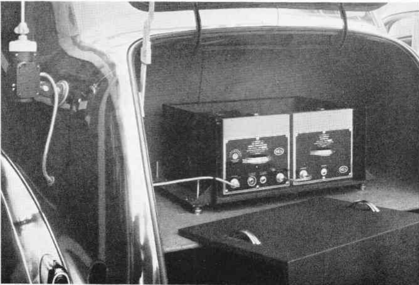
FM TRANSMITTER AND RECEIVER UNITS MANUFACTURED BY REL FOR EMERGENCY USE
