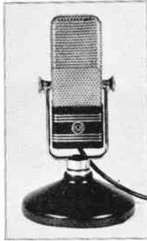
FIG. 13. RCA RATES THE 44-BX AS HAVING SUITABLE RESPONSE CHARACTERISTICS FOR USE IN FM BROADCAST STUDIOS
