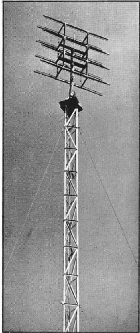
FIG. 15. THE 240-MC. RADIATOR ATOP PHILADELPHIA'S CONVENTION HALL
