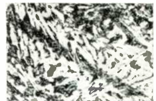
Same iron rendered malleable by heat treatment. Shows spots of nodular carbon.
