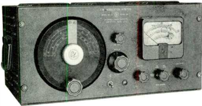
Model MD-25 Universal FM Modulation Monitor covers all frequencies from 30-50, 72-76, 152-162 mc.
