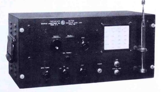
**IMPORTANT:** The accuracy of any BROWNING frequency meter can be checked in the field against WWV standard frequency signals because the crystal frequencies employed are sub-multiples of WWV. This essential feature is not found in other communications-type meters. NOTE: Use the BROWNING WWV Calibrator for precision checking.
