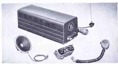
GENERAL ELECTRIC MOBILE COMBINATION MC-201 for dependable operation in the 152-162 mc band. Features single unit design with receiver, transmitter and power supply mounted mechanically on one main chassis. Electrical connection is made instantly through G-E special-design plug-in feature. MC-201 consists of receiver, transmitter, power supply, loud speaker, microphone with retractable cord, antenna, control unit, power and control cables.
