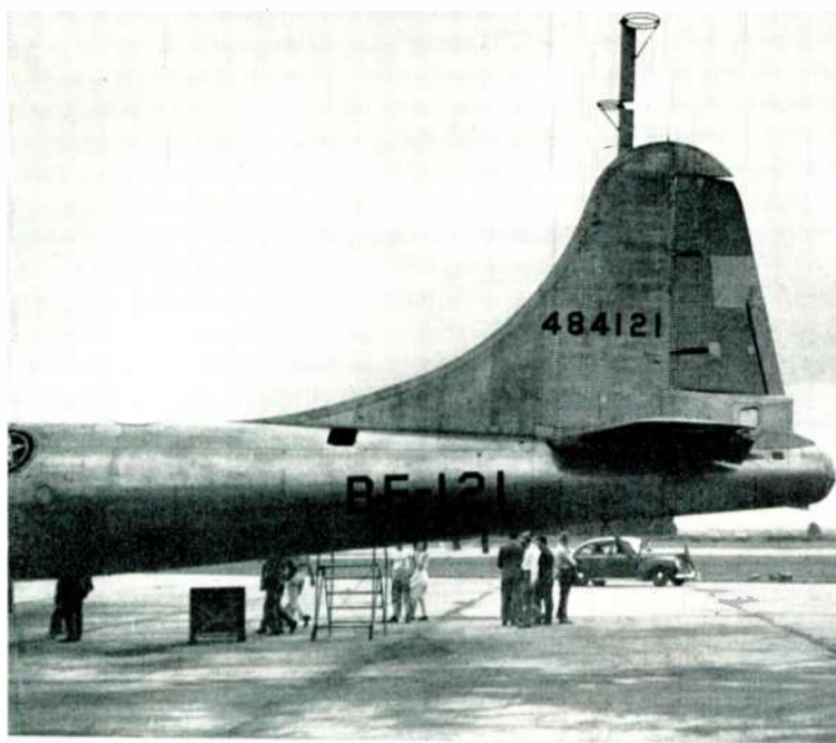
FIG. 3. This view shows receiving antennas in detail. FIG. 4. Mounting of the transmitter antenna mast. Ring antenna is for audio
