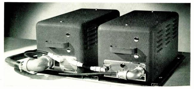
FIG. 1. FM TRANSMITTER, LEFT, AND THE RECEIVER USED IN WESTERN ELECTRIC MOBILE COMMUNICATIONS INSTALLATIONS
