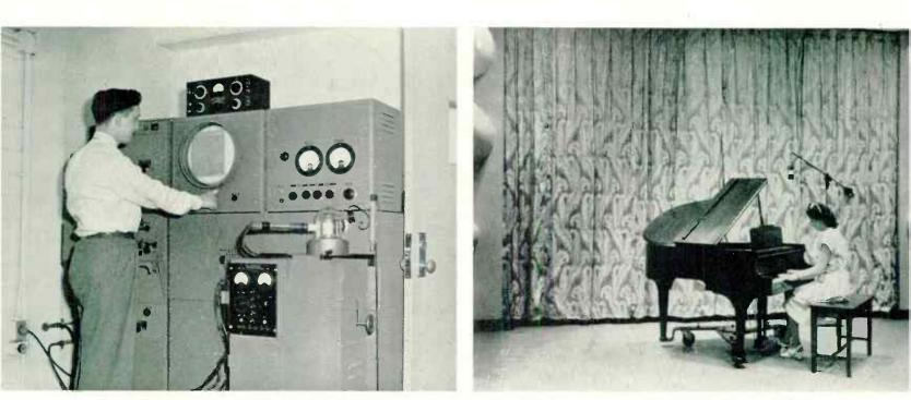
1: SPECTRORADIOMETER TESTS LUMINOUS MATERIALS FOR CATHODE-RAY TUBES 2: GLASS CURTAIN ADJUSTS STUDIO ACOUSTICS
