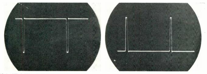
FIG. 3, LEFT: PATTERN OF THE SYNCHRONIZING PULSES GENERATED AT THE GRID OF THE MULTIVIBRATOR OR BLOCKING CON-DENSER. SUCH PULSES MAINTAIN THE VERTICAL AND HORIZONTAL PICTURE SYNCHRONIZATION. FIG. 4, RIGHT: INVERSION AT PLATE
