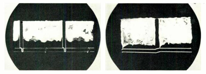
FIG. 5, LEFT: OSCILLOSCOPE PATTERN AT THE OUTPUT OF THE SECOND DETECTOR. IN THIS CASE THE 'SCOPE IS SET AT 60 CYCLES. FIG. 6, RIGHT: RESULTS WHEN 'SCOPE IS SET AT 15,750 CYCLES. STEAM-LIKE CLOUDS ARE CAUSED BY PICTURE SIGNAL
