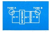
**CONDITION 2:** Carrier being modulated. Tube B, now needed, kicks in, adding its quota of power to haudle the increased load and changing the impedance so that Tube A also steps up its output. Both tubes work to full capacity and at high efficiency.
