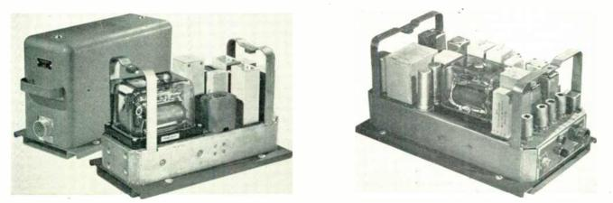
FIG. 3. LEFT: SELECTOR SET FOR USE WITH ANY MAKE OF EQUIPMENT. FIG. 4, RIGHT: SELECTOR SET ON A W.E. RECEIVER
