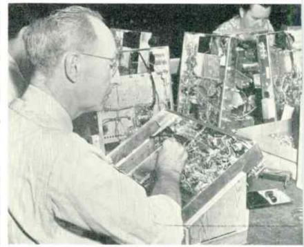
7: WORK IS DISTRIBUTED IN UNITS OF TIME, TO KEEP LINE MOVING STEADILY. 8: FREQUENT INSPECTION CATCHES ERRORS QUICKLY 9: COIL UNITS ARE ADDED HERE. 10: MOUNTING THE SHIELDS. LINES ARE PIPED FOR COMPRESSED AIR TO OPERATE SCREWDRIVERS
