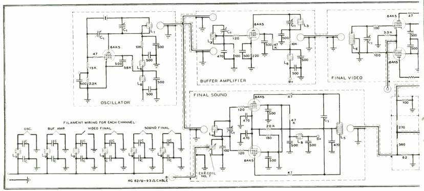
FIG. 5. THE CRYSTAL OSCILLATOR, BUFFER AMPLIFIER, AND FINAL VIDEO AND SOUND AMPLIFIERS FOR EACH CHANNEL ARE
