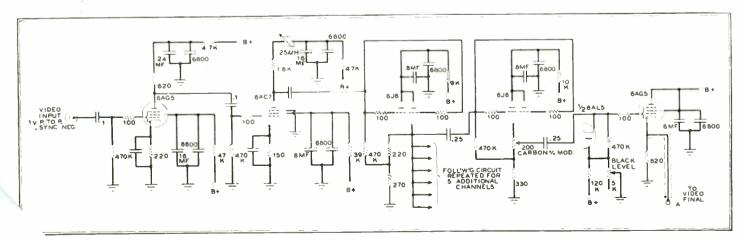
FIG. 4. THIS VIDEO AMPLIFIER CIRCUIT REQUIRES AN INPUT OF 1 VOLT PEAK-TO-PEAK, AND HAS AN OVERALL GAIN OF 6
