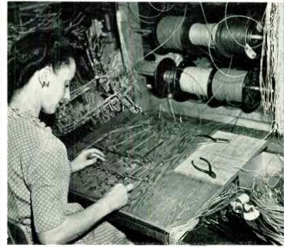
1: PRE-TESTING STOPS DEFECTIVE COMPONENTS BEFORE THEY REACH PRODUCTION LINES. 2: PRINCIPAL WIRES ARE CABLED 3: RIVETS REPLACE SCREWS AND NUTS FOR MOUNTING COMPONENTS AND HARDWARE. 4: ADDITIONAL RIVETING OPERATIONS
