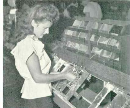
5. SWITCH SECTION SUB-ASSEMBLY IS WIRED BEFORE IT IS MOUNTED ON CHASSIS. 6: CHASSIS STARTS ON MAIN ASSEMBLY LINE
