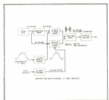
FIG. 2. BLOCK DIAGRAM OF THE VIDEO-AUDIO SIGNAL GENERATOR.
