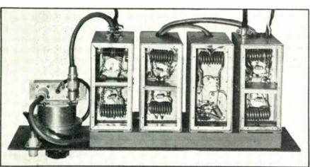
FIG. 6. ONE OF THESE SEPARATE RF ASSEMBLIES IS USED FOR EACH CHANNEL
