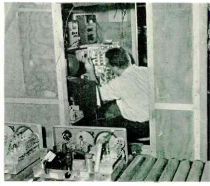
13: FINISHED CHASSIS ROLL TO THE TEST CAGES. 14: LONG PRACTICE AND GOOD INSTRUMENT SPEED FIVE-BAND ALIGNMENT 14, 15: NO REPAIRS ARE MADE IN THE CAGES, FOR A FAST PACE MUST BE MAINTAINED, 16: APPROVED CHASSIS, READY FOR PACKING
