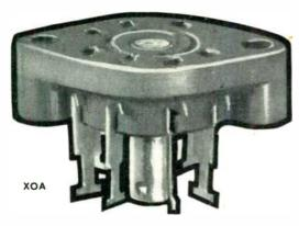
● The XOA Socket for Miniature Button 7-pin bases is mode of low-loss mico-filled bokelite. It mounts with two 4-40 screws. Terminols for the Type XOA extend axially from the socket. Type XOR is identical to Type XOA, but has terminals extending radiolly. Short heavy terminols reduce contact inductonce. Lawer effective capacity between terminols reduces circuit capacity.
