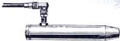
This is a Dielectric Antenna, with special directional properties for radar.
