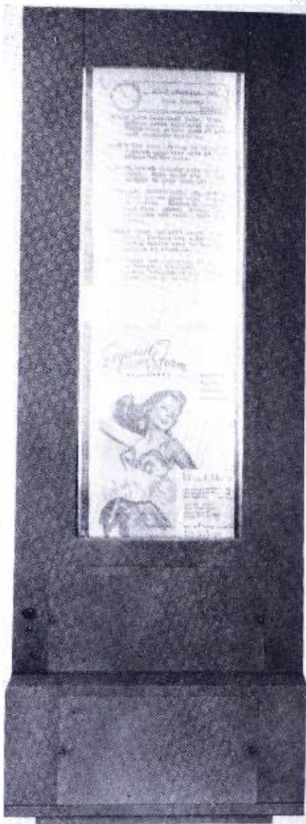
FIG. 3. BULLETIN BOARD RECORDER GIVES 4 TIMES ENLARGEMENT
