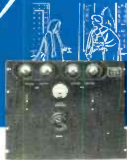
1928. This ac operated amplifier, one of the first made, reduced maintenance costs and did away with cumbersome batteries and charging equipment. It was used to record some of the earliest sound motion pictures.
