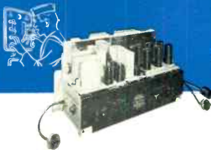
1942. This compact and powerful unit for battle announce systems is typical of Western Electric amplifiers designed during the war. It operated dependably when mounted a few feet from the largest guns.
