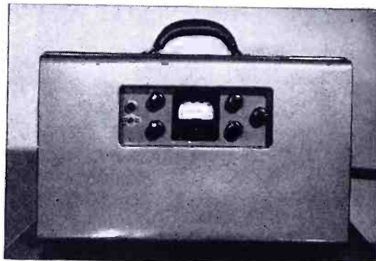
FIG. 12. TRANSMITTER CONTROL UNIT IN PORTABLE CARRYING CASE
