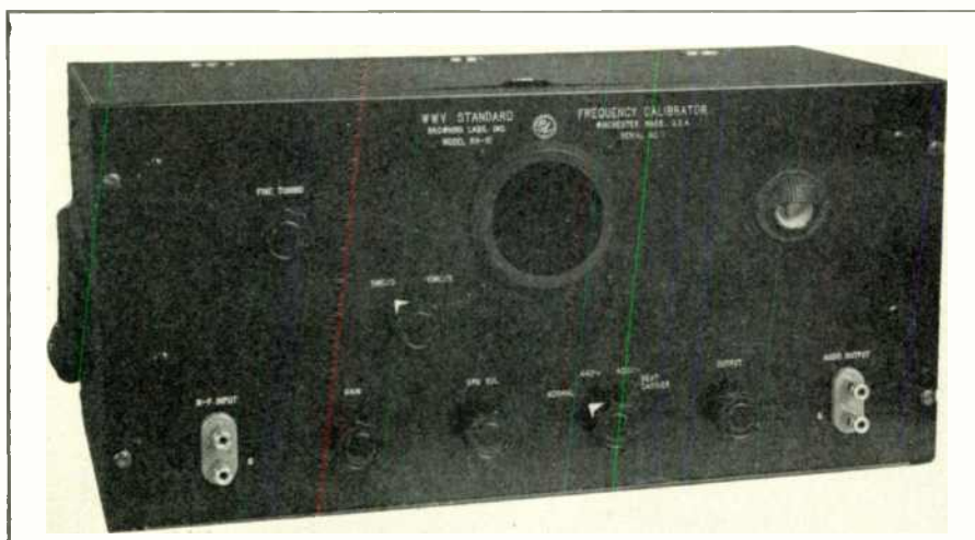
FIG. 2. RADIO CIRCUITS ARE PROVIDED FOR 2.5 AND 5 MC., 5 AND 10 MC., OR 10 AND 15 MC.
