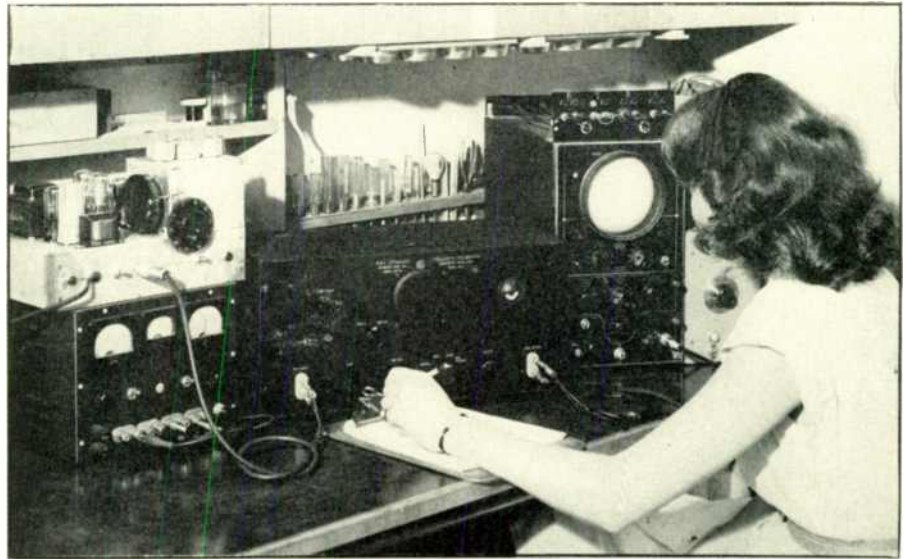
FIG. 1. THE CALIBRATOR SETUP FOR THE TEST POSITION OF A PRODUCTION LINE
