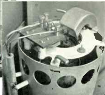
Amplifier tank assembly (right half of unit at left)—Visible are outer conductor of concentric-line plate tank, cathode transmission line at left, and motors to adjust cathode line, plate tank, and output coupling loop. Close-up below shows the RCA-7C24 in position, grid and filament connections, and air scoop to cool tube seals.
