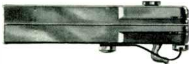
PARTIAL VIEW of cartridge, showing knee-action Nylon needle and metal needle guard. The cushioning action of Nylon affords additional protection for the sapphire stylus.
