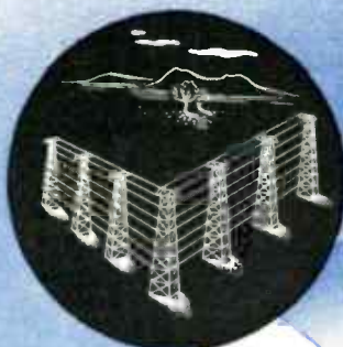
1929 Curtain antennas developed for beaming short-wave radio telephone messages to Europe and South America ... improved commercial service.
