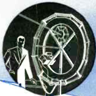
1920 Loop antenna for 400-500 meter ship-to-shore radio telephone receivers. Its design enabled earliest measurements of field strength.
