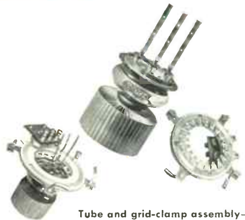
Tube and grid-clamp assembly —The new RCA-7C24 (top) is a forced-air-cooled triode especially developed for Grounded-Grid circuits. (Plate dissipation: 2 kw at frequencies up to 110 mc; power output: 4 kw at 110 mc, class C service.) The flange ring at the top of glass envelope is the grid terminal. The grid support is conical in shape and extends well into the tube to provide complete shielding between filament and plate circuits. The circular grid clamp (right) is used to make connection to the disk-seal flange of the grid. With the tube and grid clamp in position (above, left), plate and filament circuits are effectively isolated and a direct, low-inductance path is provided to the grid. No neutralization is needed.
