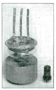
FIG. 11. SIZE COMPARISON BETWEEN THE 7C24\_AND A STANDARD METAL 6AC7
