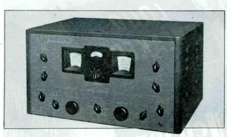
FIG. 1. HAMMARLUND COMMUNICATIONS RECEIVER FOR .54 TO 31 MC.
