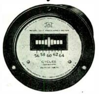
Size-31/4" flange, dull black metal case for flush panel mounting. 9 or 11 reeds, full or half cycle increment. Reed in resonance vibrates as shown. Simply READ THE REED, and that's your fre-
