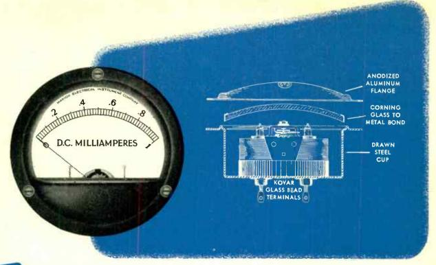
They're totally sealed. The Marion design and glass-to-metal sealing process assure true hermetic sealing. And the bond between the metallized glass rim and the steel case is capable of withstanding extreme thermal shock.
