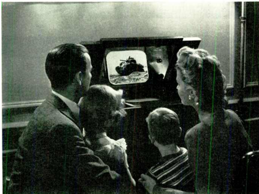
FIG. 1. PREWAR RCA MODEL WITH 12-IN. TUBE PRODUCED AN IMAGE 7 BY 10 INS.
