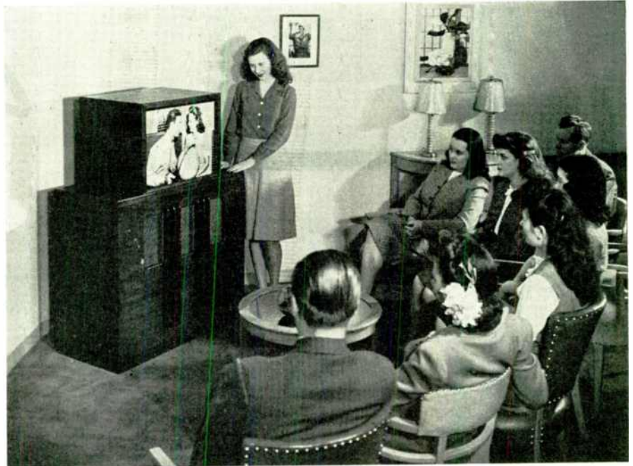
FIG. 2. NEW RCA OPTICAL SYSTEM PRODUCES IMAGE 16 BY 21 INS. FROM 5-IN. TUBE
