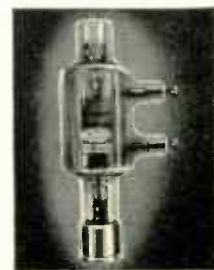
ML-500, a high-frequency triode. Maximum plate dissipation 500 watts with full power input at frequencies up to 50 megacycles.
