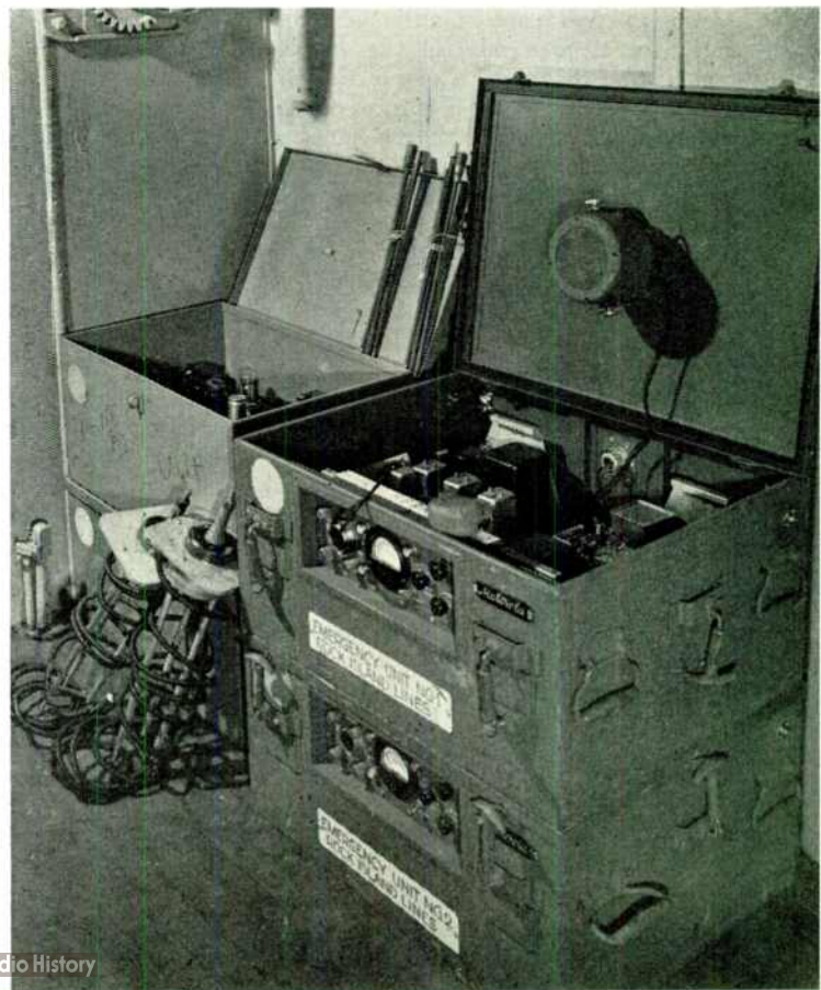
FIG. 8. TRUNK-MOUNTED FM UNITS, WITH PORTABLE ANTENNAS ARE USED TO PATCH LINES BROKEN BY STORMS
