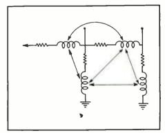
FIG. 3. ILLUSTRATING MUTUAL INDUCTANCE BETWEEN ELEMENTS OF ATTENUATOR
