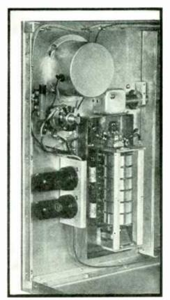
FIG. 13. ASSEMBLY OF ATTENUATOR AND SWITCH ELEMENTS SHOWN IN FIGS. 11 AND 12
