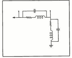
FIG. 2. ELECTRICAL EQUIVALENT OF ONE STEP OF CONVENTIONAL ATTENUATOR
