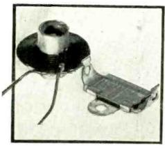
FIG. 14. ACTUAL SIZE OF THE RF FILTER CHOKE AND CONDENSER IN SUPPLY LEADS
