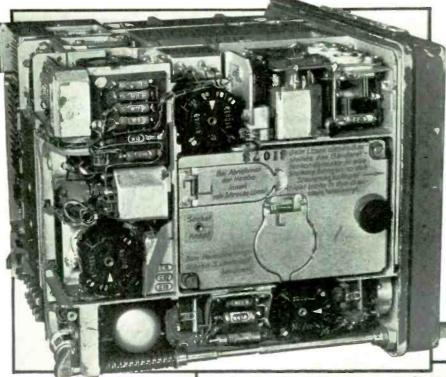
FIG. 3, ABOVE, IS LEFT SIDE. IT IS SURPRISING TO SEE SIMILARITY BETWEEN AMERICAN AND GER-MAN COMPONENTS. NOTE THE CLOSE-FITTING COVERS ON THE LARGE SHIELD PLATE, BASES OF TWO TUBES CAN BE OBSERVED IN THIS PICTURE
