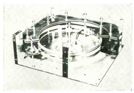
FIG. 6. THE COMPLETE OSCILLATOR ASSEMBLY, WITH ONE SIDE FLATE REMOVED. THE MAIN SHORTING CONTACTS ARE STATIONARY, WHILE THE UNIT IS ROTATED
