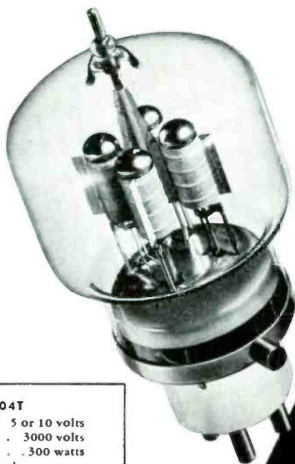
Before filaments are sealed into the triode they are placed in a temporary vacuum where they undergo their first emission test. Thus faulty filaments may be weeded out without further processing.
